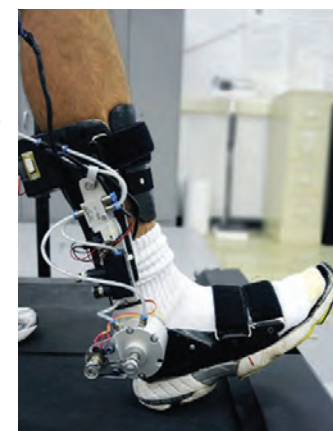
Early generation PPAFO prototype Courtesy Georgia Institute of Technology
